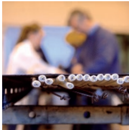
Cable mounting for large scale fire test
