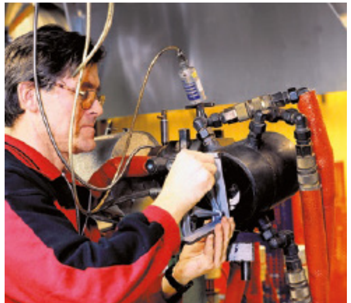
Adjustment of extruder die
