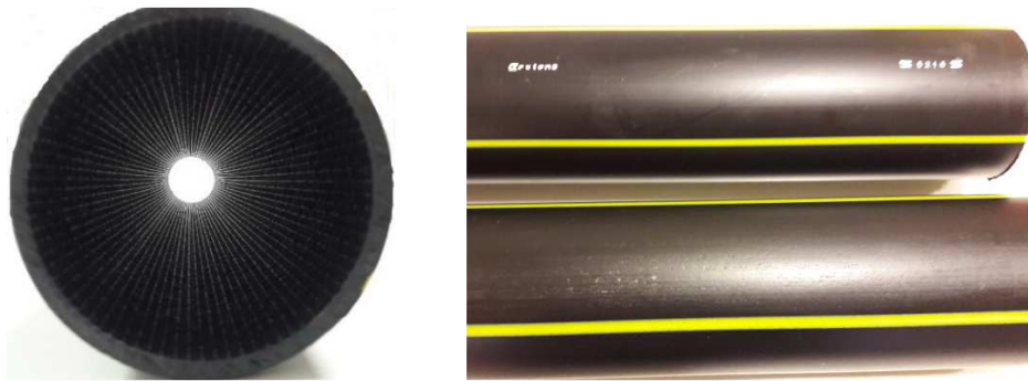
Figure 56 Pipe produced with 10 % (1 mm) XLPE in HDPE.
