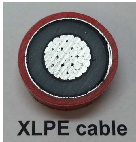
Figure 1 Cross-section of the PP-TPE Cable Figure 2 Cross-section of the XLPE Cable
