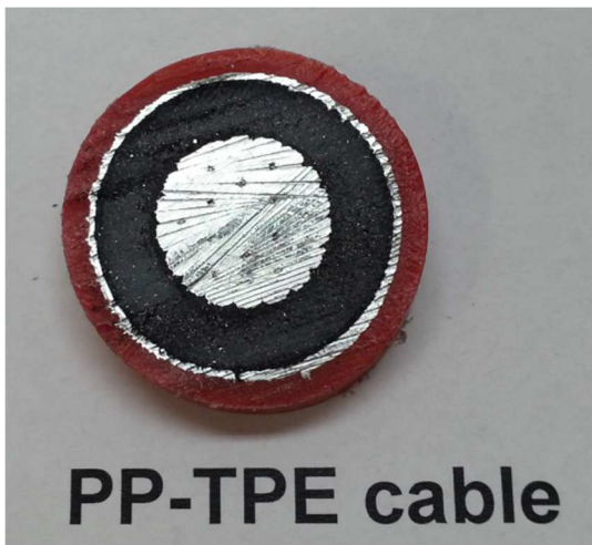
Figure 1 Cross-section of the PP-TPE Cable Figure 2 Cross-section of the XLPE Cable
