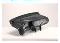
Borcycle™ GE2331SY is a 20% glass fiber reinforced PP compound containing 40% PCR. Intended for use in injection molding of non-visible interior parts like instrument panel or center console carriers, GE2331SY fulfills premium OEM emissions, fogging, and odor requirements.
