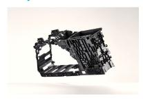
Borcycle™ GD3600SY is a 30% glass fiber reinforced PP compound containing nearly 70% PCR polymer. Intended for use in injection molding of non-visible parts like center console carriers, GD3600SY offers an excellent stiffness/impact balance while maximizing the use of recycled polymers.
