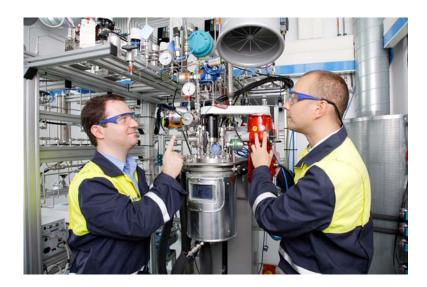
The new reactors are being used for PE polymerisation. The first test samples were produced. (Alexander Krajete, Michael Benisch)
