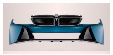
Developed in cooperation with BMW for the front bumper of the electric sports car BMW i8, Daplen™ EE112AE is a recent and specific example of how Borealis and Borouge innovations can play a role in facilitating systematic lightweight construction in the automotive industry.
